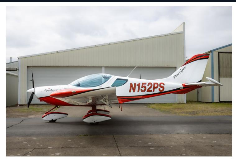
Need a Light Sport aircraft? This sleek looking factory built 2010 LSA features a 100hp Rotax 912 ULS2 engine. 1674 TT, Dynon EFIS-D100, Dynon EMS-D120 Engine Monitor, Dynon Autopilot, Garmin 696 GPS, Garmin GTX-330 Transponder, Garmin GDL82 ADS-B Out, Garmin SL30 Nav/Com, PS Engineering Intercom. Avionics Master. Safety equipped with BRS parachute. Trickle Charger, Canvas Cover
