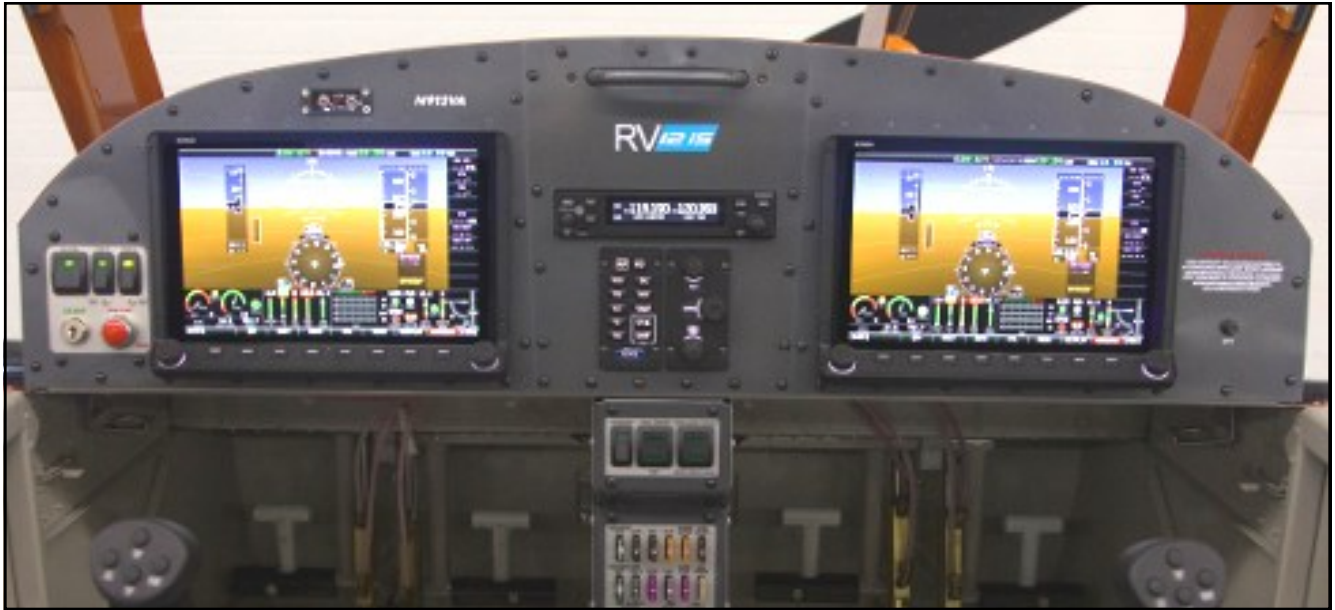
INSIDE THE PREMIUM CABIN: A modern glass panel, featuring the Dynon Skyview HDX with Autopilot Button and Knob modules and a Garmin GTR 200 comm radio/ intercom.
