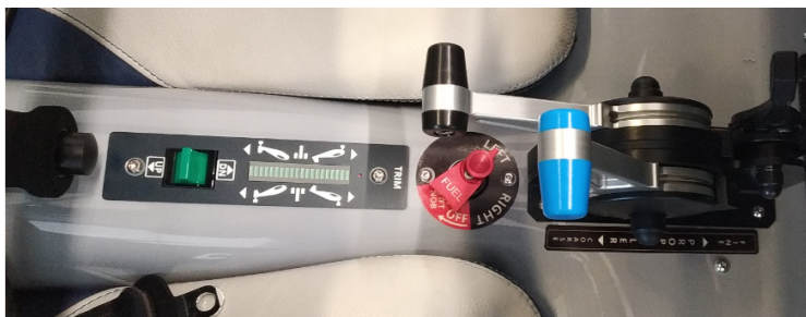
Typical center console arrangement (view of: throttle quadrant, fuel selector, elevator trim, flap lever)
