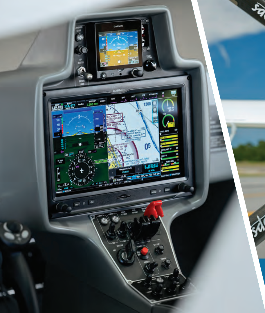
A Garmin G3X PFD/MFD with engine gauges and G5 standby instrument provide exceptional situational awareness. The lower wing of the biplane design protects the five-blade, fixed-pitch, composite propeller from spray during water takeoffs and landings.
